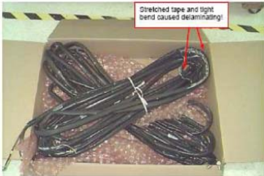
Figure 2. Stretched Tape Delaminating
