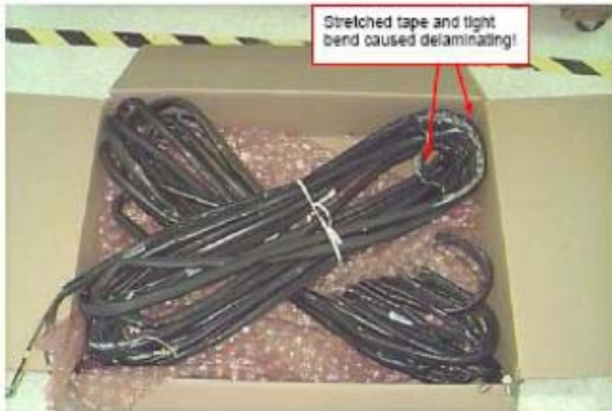
Figure 2. Stretched Tape Delaminating
