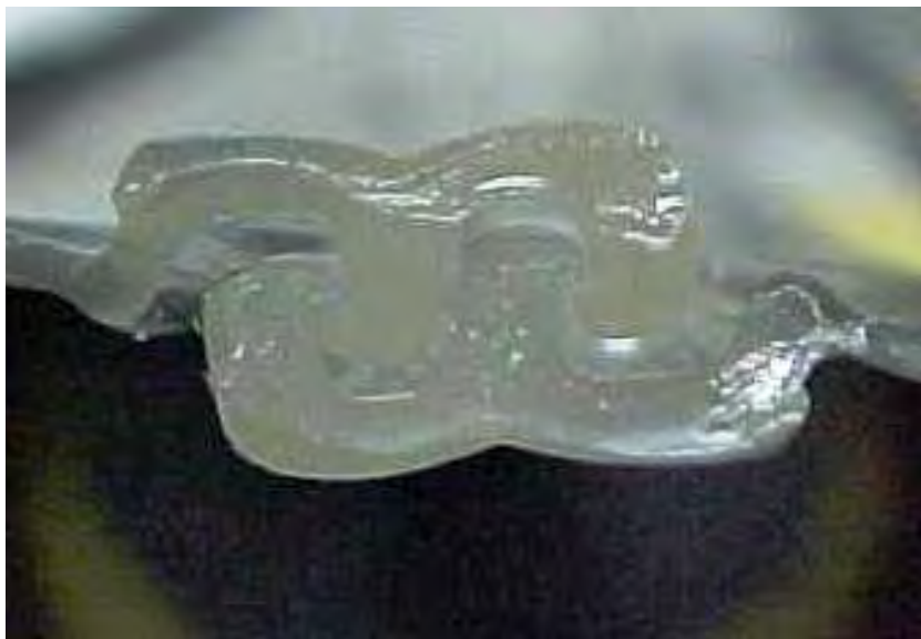
Photo 3. Correctly aligned and inter-locked track halves
