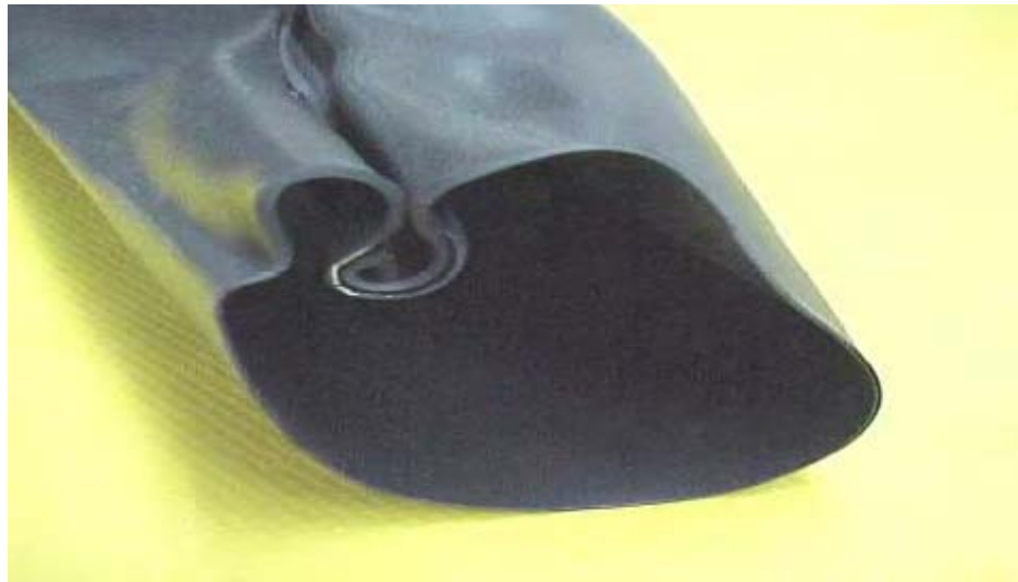
Photo 6: Overlap seams “U” shape curl prior to full shrinkage.
