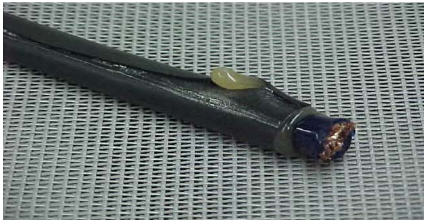
Photo 15: Seam rupture; too much heat, too fast!
