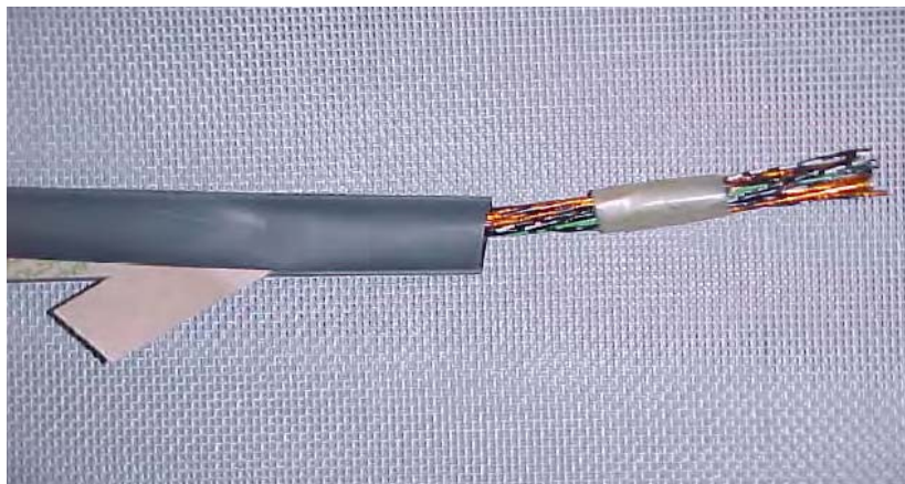
Photo 3: PRT closed around wire bundle
