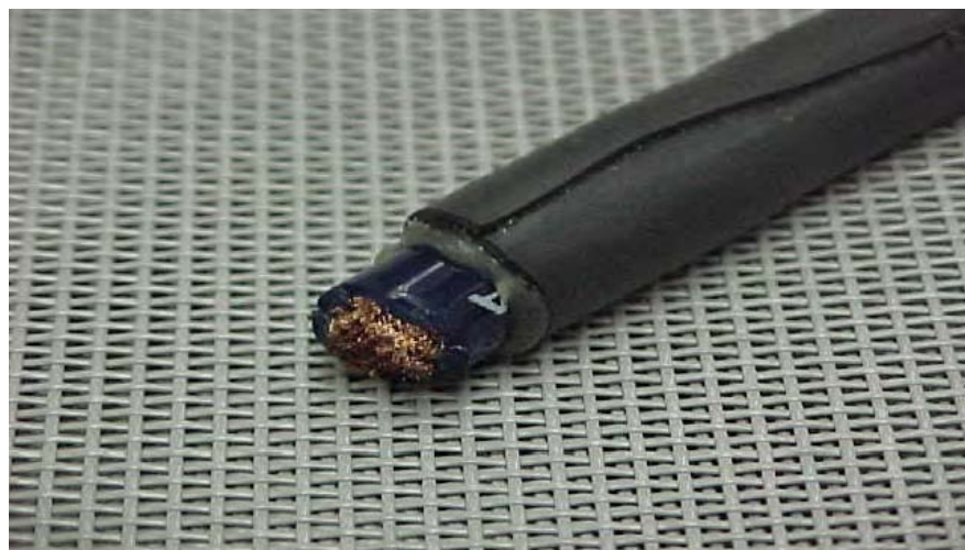
Photo 11: Fully shrunk PRT with good Z-Block adhesive fillet
