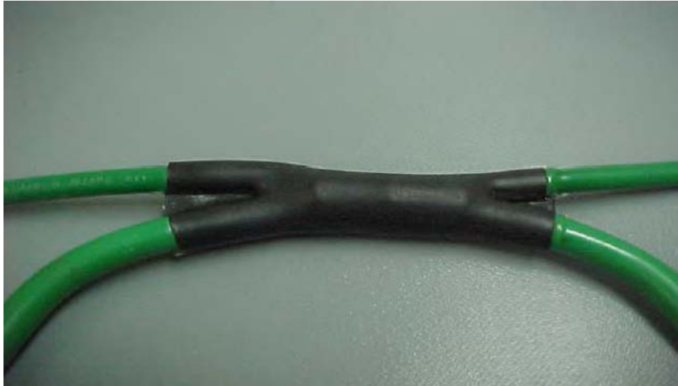
Photo 13: Typical four legged splice breakout
