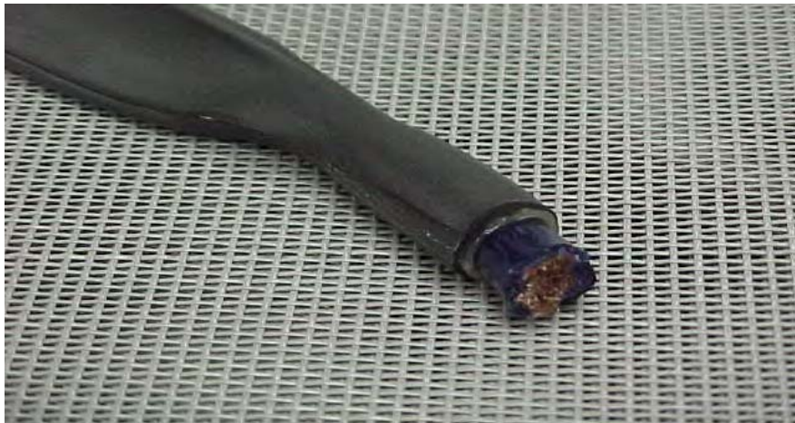
Photo 10: PRT tubing shrunk down on to Z-block tape
