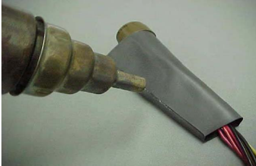
Photo 2: Heat gun with reducer nozzle
