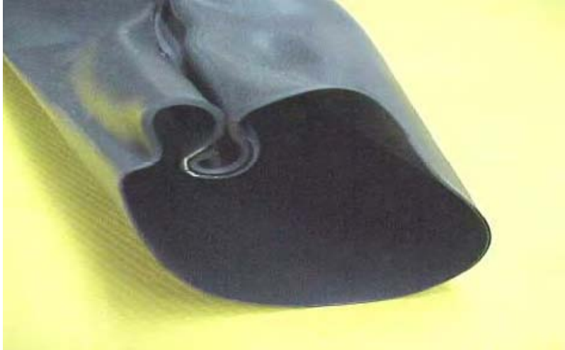
Photo 3: Adhesive overlap seam curling into a “U” shape
