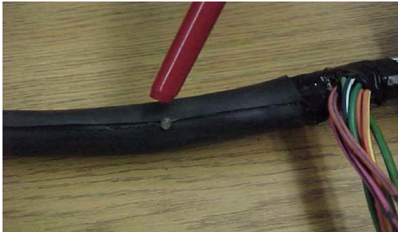
Photo 4: Adhesive ball removed with thumb pressure
