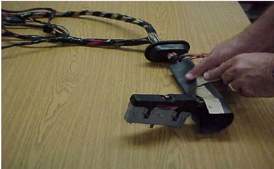
Photo 1: Installing PRT™ around cable.
