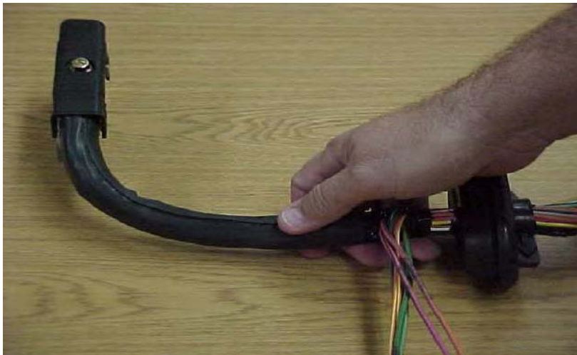
Photo 4: Rubbing adhesive seam after shrinking.
