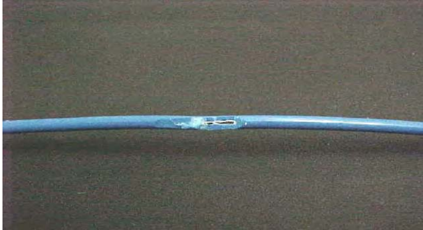
Photo 1: Typical wire insulation damage
