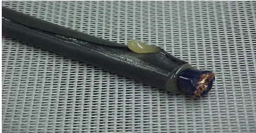
Photo 6: Typical overlap seam rupture
