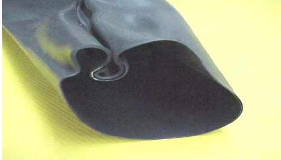
Photo 5: Overlap seams curled up prior to full shrinkage.
