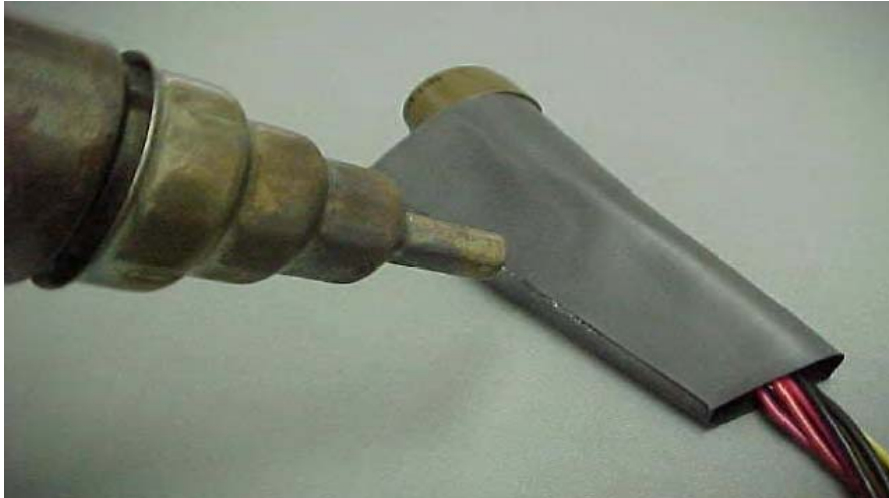
Photo 4: Nozzle focused near tubing center on overlap seam
