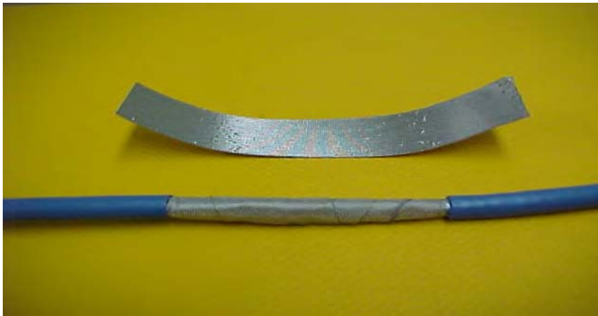
Photo 7: Finished shield braid repair.
