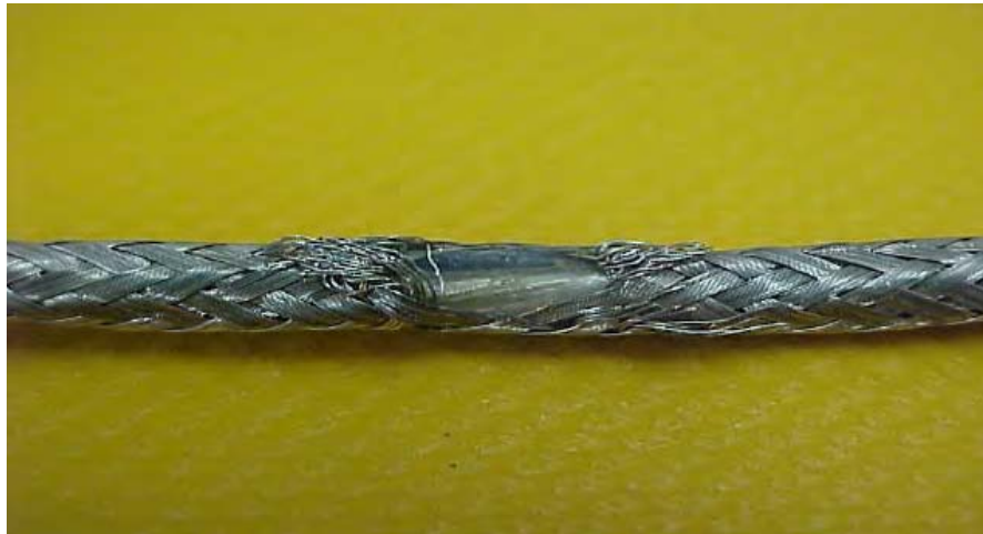
Photo 5. Broken shield strands dressed back smoothly.
