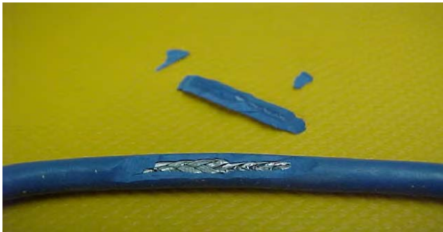
Photo 3: Damaged insulation removed.
