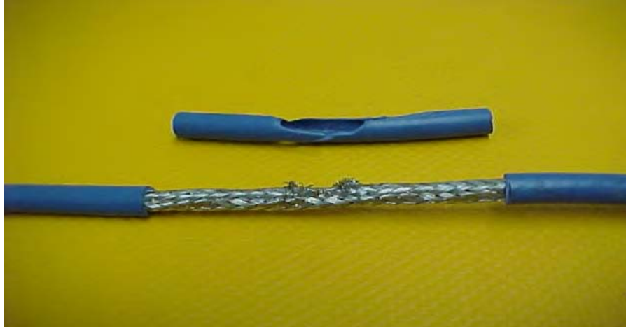
Photo 4: Insulation removed around braid damage
