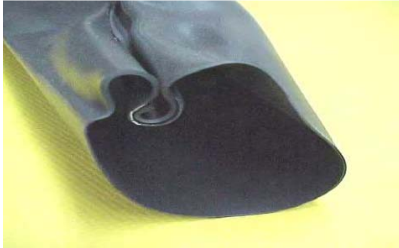
Photo 10: Overlap seams curled up prior to full shrinkage.
