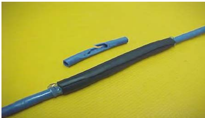
Photo 11: Finished PRT-1553 jacket with good adhesive fillet
