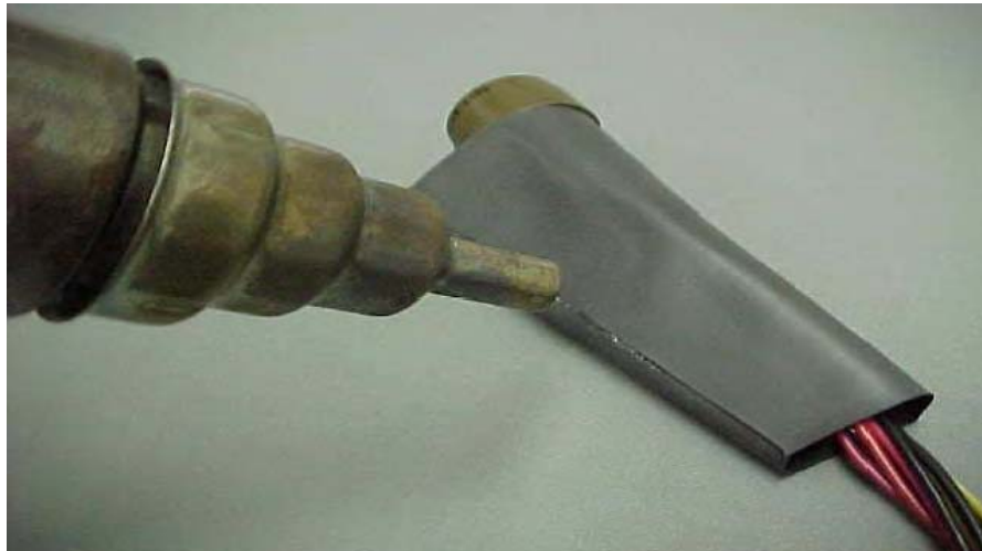
Photo 9: Reducer nozzle on heat gun.
