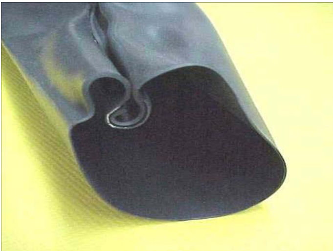
Photo 15: Overlap area curled up upon heating
