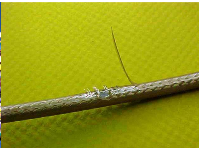
Photo 2: Minor shielded cable damage
