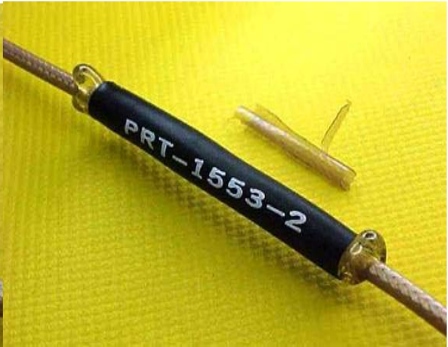
Photo 10: Finished RG-180 repair test cable
