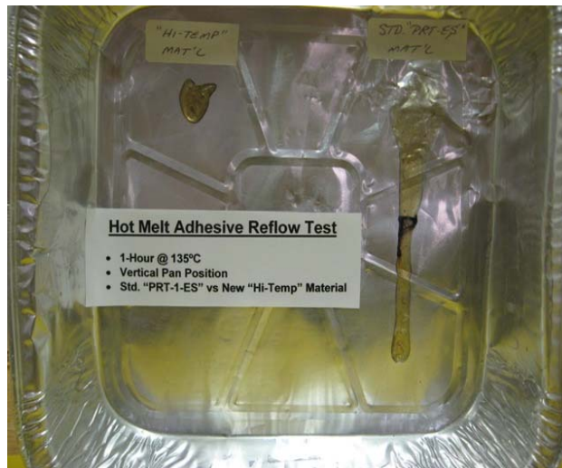
Photo 2: Vertical Tray (1-Hour @ 135°C)
