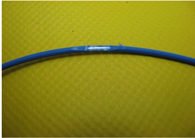
Photo 6: Simulated wire insulation damage
