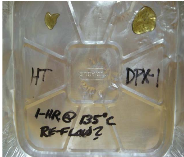
Photo 1: Horizontal Tray (1-Hour @ 135°C)
