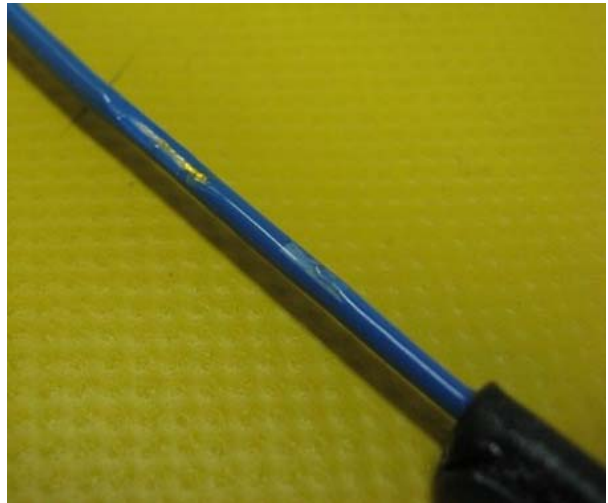
Photo 10: ES slippage (4-Hr @ 135°C)
