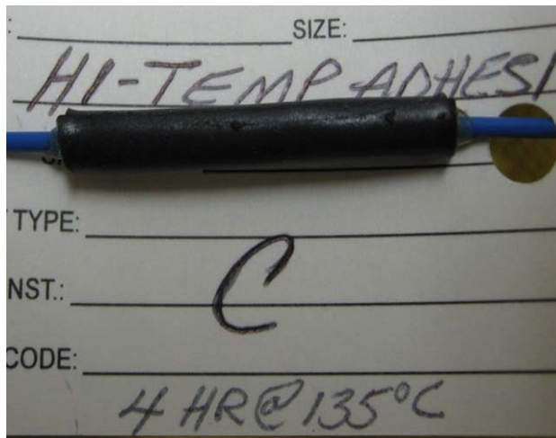
Photo 11A: HT sleeve (4-Hour @ 135°C)
